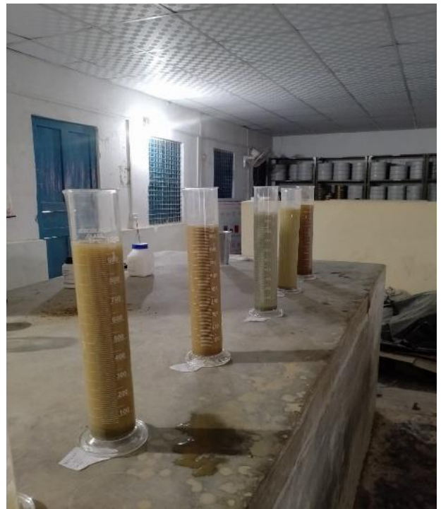
Figure E1: Photograph Showing Hydrometer Testing in Laboratory
